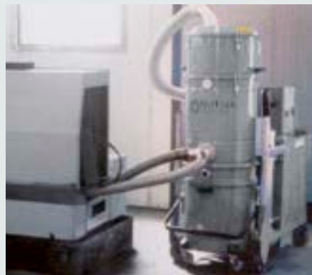
Fixed application for recovery of graphite
