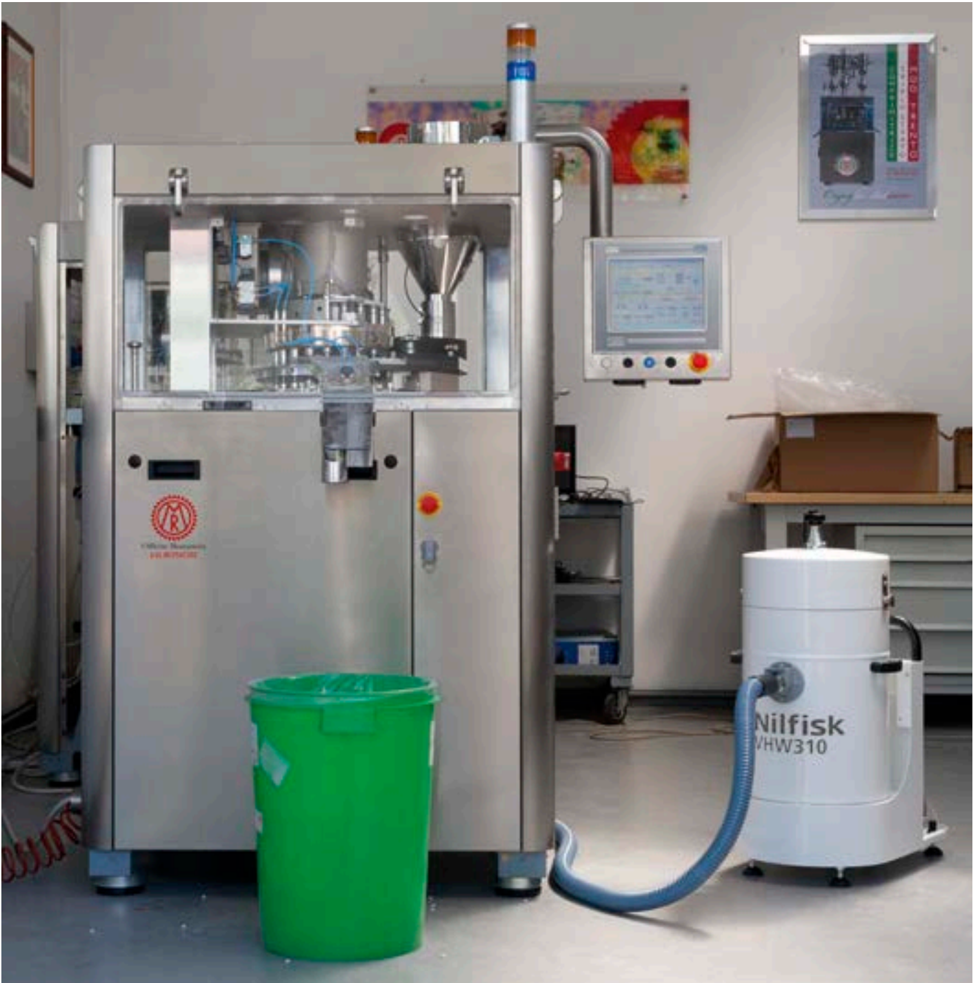
Fixed vacuum on tablet press machine.
