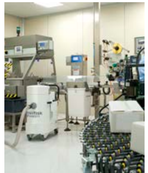
Recovery of waste from a packaging machine.
