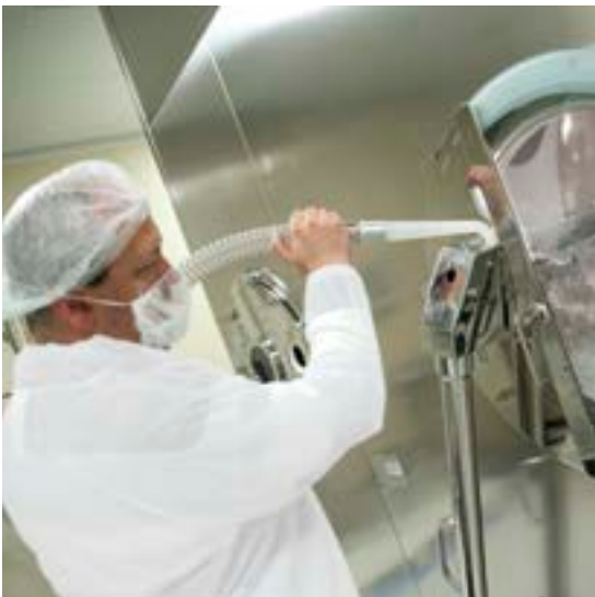
Cleaning of a coating pan.
